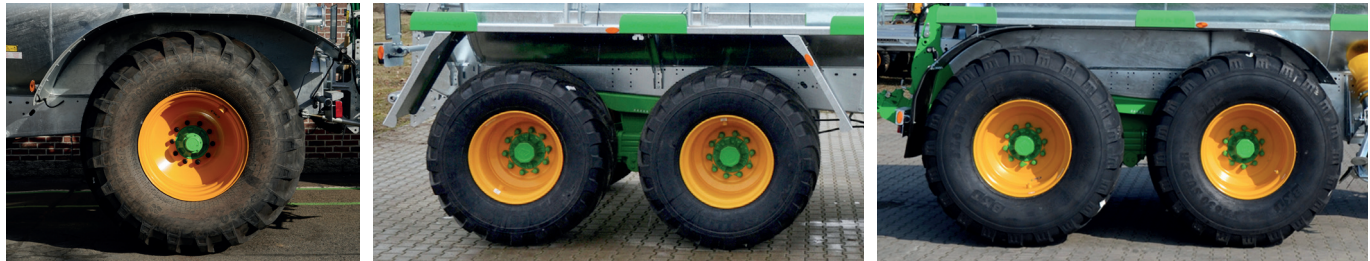
Wheel recesses on single and double-axle machines with several options possible
