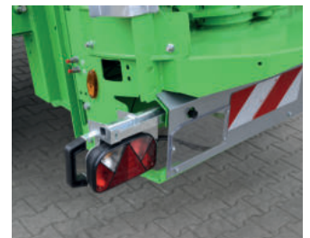
Feux de signalisation full LED escamotables
