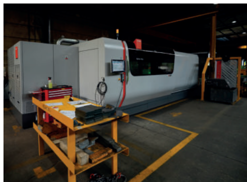
15 kW optical fibre laser for ultra-fast cutting of steel sheets with minimum overheating to minimise distortion
