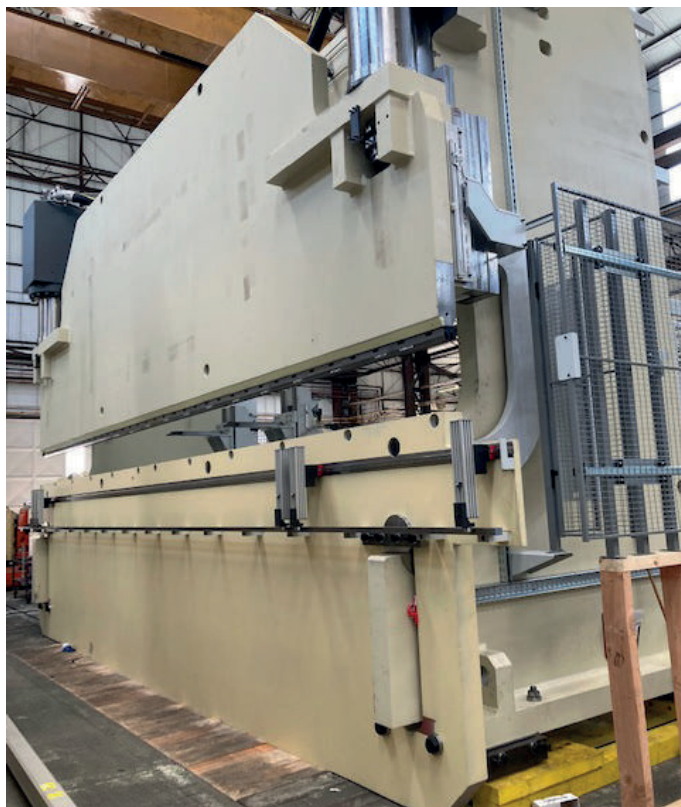
New press brake being assembled at the supplier (left) and its future location in the factory (right)
