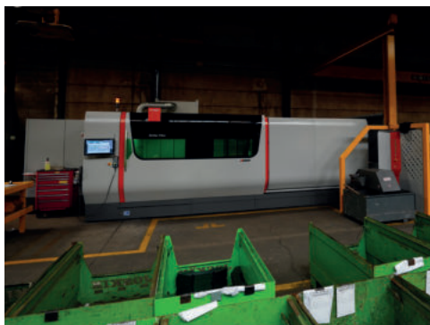
15 kW optical fibre laser for ultra-fast cutting of steel sheets with minimum overheating to minimise distortion
