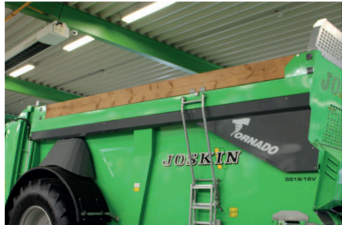
Wooden or aluminium extensions (250 mm) to increase the loaded volume
