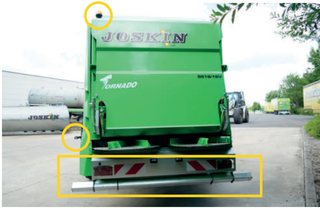
Rear bumper, extra lighting (flashing beacon, lights, etc.)
