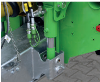
Simplified hydraulic drawbar suspension with closed circuit
