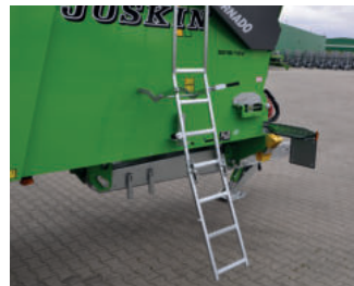
Galvanised access ladder
