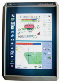
Control of the hydraulic functions of the spreader through Load Sensing or ISOBUS
