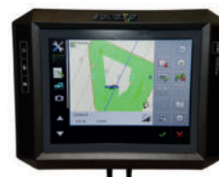
Control of the hydraulic functions of the spreader through Load Sensing or ISOBUS
