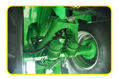
articulated triangular structure. Already successfully used on dump tipping trailers, this suspension type allows to better follow the ground, whatever its topography, as well as a higher maintenance ease (lubrication, etc.).
