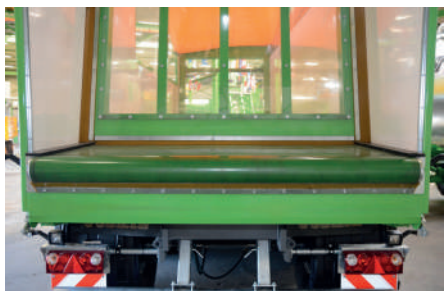
Conveyor belt over the entire width of the machine
