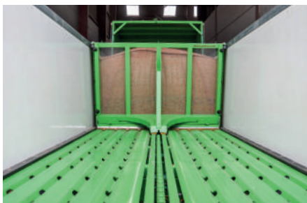
Ribbed and perforated floor
