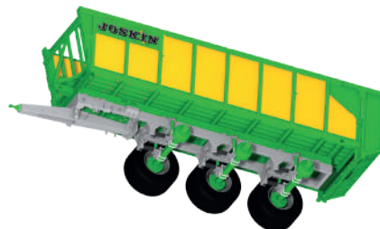
Hydro-Tridem running gear
