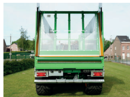
Transparent front wall for a better visibility from the cabin
