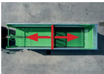
Mobile front wall pulled by the conveyor belt to the rear of the machine
