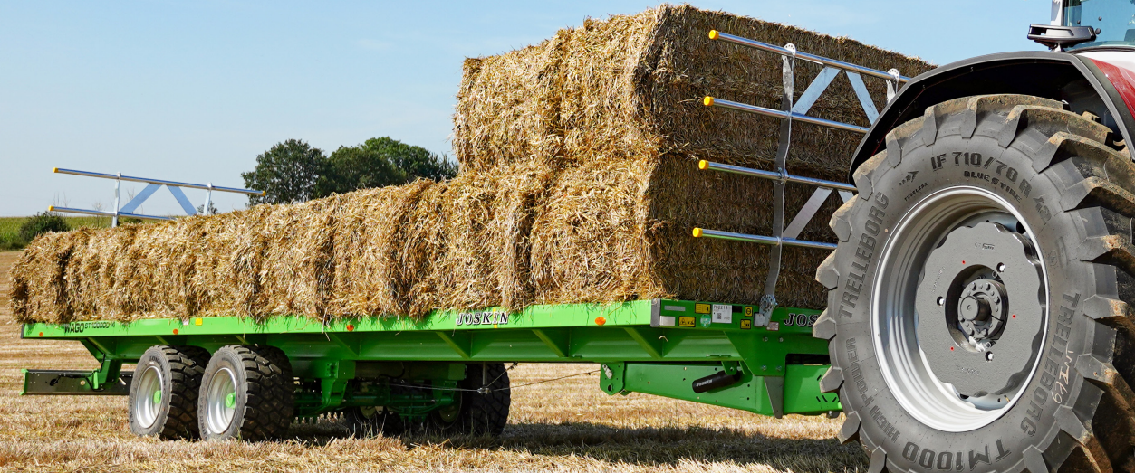
Floor in galvanised folded steel sheet or painted chequered plate
