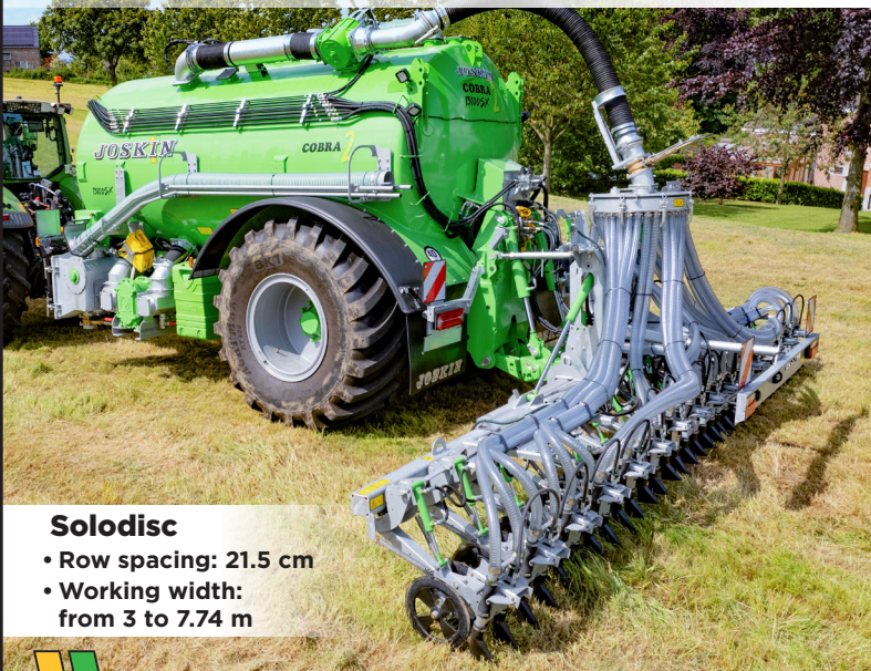
Self-sharpening discs (400 x 20 mm) on hubs with "lifetime lubrication"
