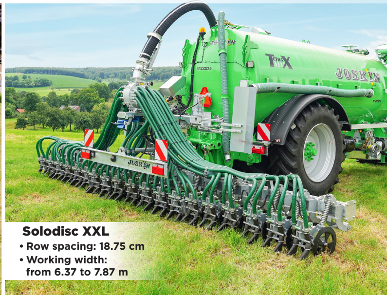
Fully galvanised frame with pendulum system
