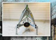
Large-diameter (1 3/4" - 50 mm) transmission shaft with 55 mm bearing
