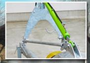
Single-acting cylinder to adjust the angle up to 45°
