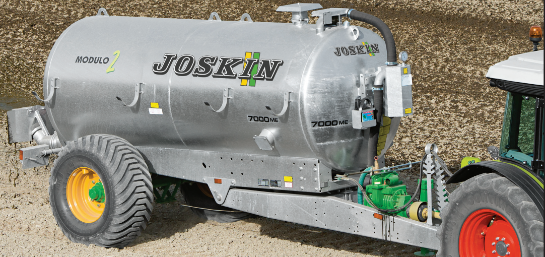
Autonomous filling and emptying with a vacuum pump
