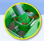
Telescopic tipping cylinder with double oscillating frame positioned forward in the chassis
