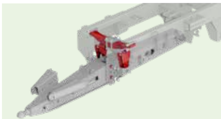
Drawbar with mechanical suspension (with cross spring leaves) on double-axle models.
