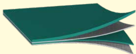
Conveyor belt structure: 4 layers of fabric and PVC with nylon reinforcement, the bottom layer being more resistant to friction.
